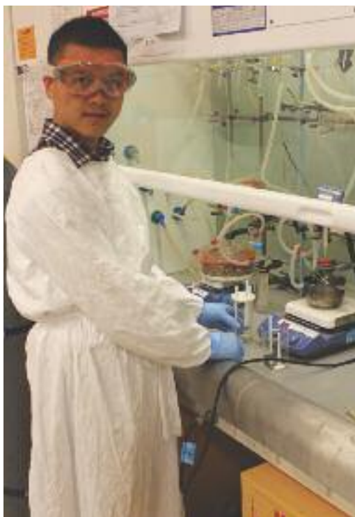
Dr Fangyang Liu performing buffer layer growth using a Chemical Bath Deposition method.
