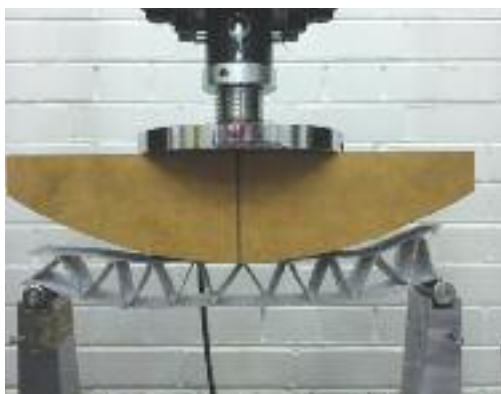
(a) Testing 2D panels for buckling failure.
