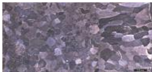
Grain refinement in Fe-4Si through \text{LaB}_6 : (a) base alloy without additions
