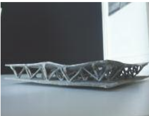
(b) Buckled 3D panel under bi-axial bending.
