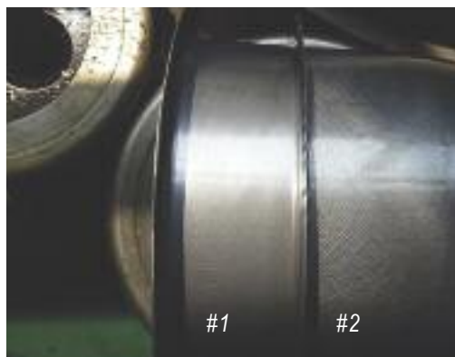
Improved ridging outcomes for Baosteel FSS 430, with #1 showing the effect after optimising alloy design, rolling and annealing processes and #2 showing the product before optimisation
